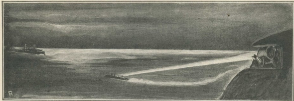
The heat waves, as well as the light waves, of an ordinary searchlight may be used to control the speed and direction of a torpedo. This illustration shows a torpedo, equipped with sensitive heat detectors, being guided by a searchlight situated on the shore.
