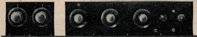
Panel view of the short-wave adapter and a standard receiver. Only the dials of the adapter are used in tuning the combined sets.
