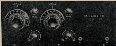
Front view of the three-tube Rasla. The first large dial is for the antenna tuning and the second for tuning the radio-frequency transformer.
