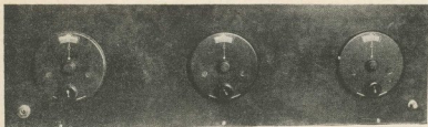
The front of panel is well balanced as can be seen above. The latest vernier type dials are used to obtain careful tuning adjustment.
