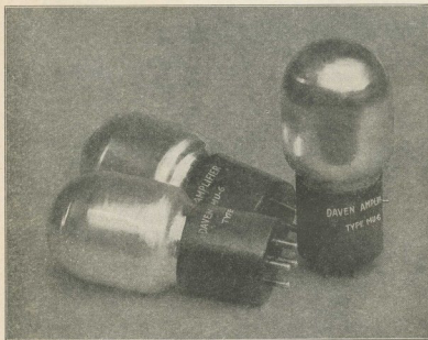
Above is shown three tubes which are especially designed for use in a resistance coupled amplifier. The one standing upright is a power tube for the last stage.
