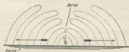
This illustration shows how the radio waves are imagined to pass over the earth's surface from a transmitting aerial.
