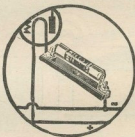
Schematic diagram showing how Amperite is connected in the filament circuit of a vacuum tube.
