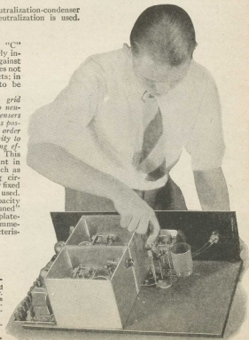
How shielding is employed in a tuned R.F. receiver. The top of the shield is removed to show construction, which is illustrated also on page 69. Photo courtesy of Hammarlund Mfg. Co.
