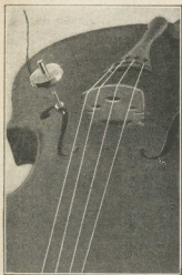
Showing detail of mounting in f-hole of violin, which does not mar instrument. With some stringed instruments it may be desirable to drill a small hole to accommodate the screw to which the microphone reed is soldered.
